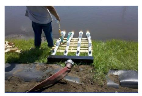
When used correctly the Floctopus<sup>™</sup> and the proper LIPVACS PAM logs will reduce turbidity and improve water quality safely without harmful toxins or chemicals. You should expect to operate the Floctopus<sup>™</sup> for several days depending upon the water condition.
